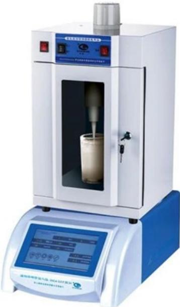
*Some integrated systems provide noise and aerosol protection.*
